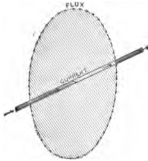
FIG. 28.—DIAGRAM OF RELATIVE DIRECTIONS OF MAGNETIC FLUX AND ELECTRIC CURRENT.
